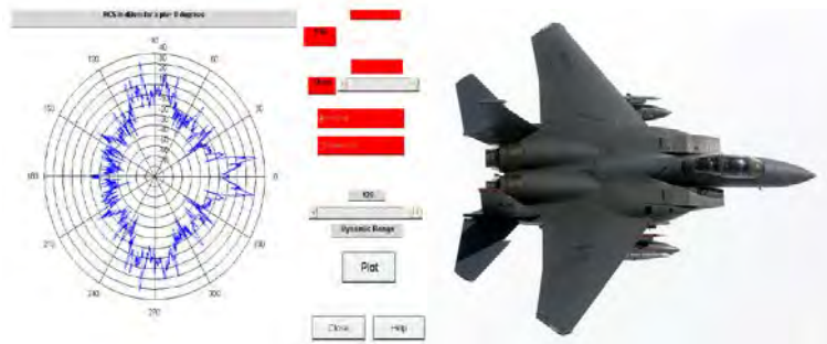
Fig. 3. Normalized cross section data of the F-15 aircraft
