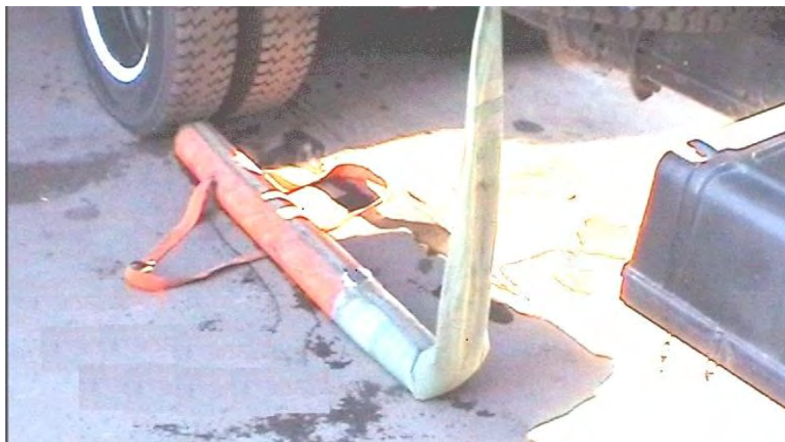
Pic. 4. The displacement of liquid by the vehicle wheel of an elastic reservoir
